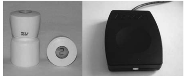
• FIGURE 47.1. MEMS (Medication Event Monitoring System) SmartCap Contains an LCD Screen; MEMS Reader Transfers Encrypted Data From the MEMS Monitor to the Web Portal. (Published with permission of MWV Healthcare/Aardex Group, www.aardexgroup.com .)
