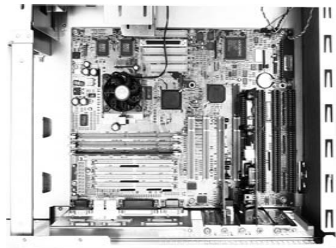
• FIGURE 2.2. Motherboard with CPU, Chips, and Slots. (Reproduced, with Permission, from Michael Alan Baxter)
